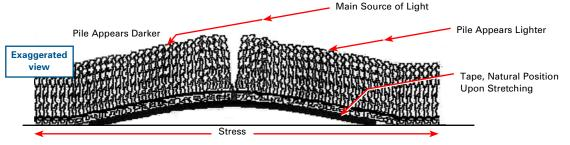
To verify that an apparent shade difference is caused by seam peaking, the seams should be viewed with a powerful overhead light while all side lighting is eliminated. When conducting such a test on a cut pile carpet, ensure that the pile is brushed in a consistent direction on both sides of the seam.
